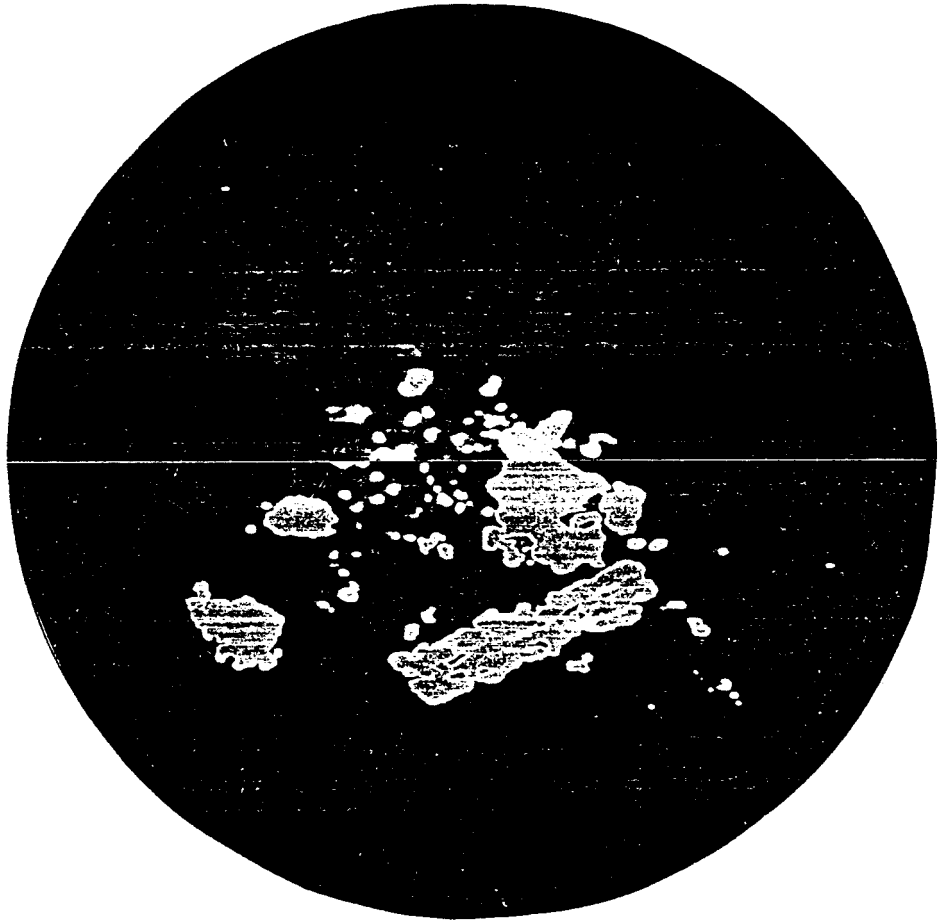
Figure 5. measurement of oxide level by application of thresholds: 6 %
