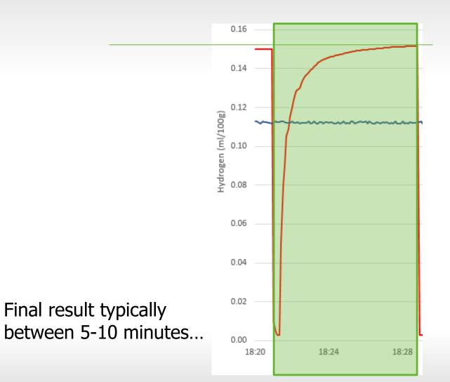
Final result given when 'gradient' stable <0.003ml/100g/min...
