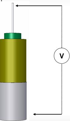
...dependent on ratio of pH<sub>2</sub> between internal and external of sensor
