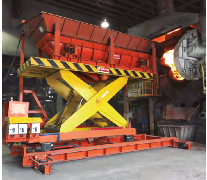
Rotary furnace charger
