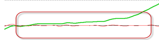
Fig. 7. This is the eutectic portion of a 95% nodularity ductile iron thermal analysis curve with the rate of cooling in green, and the 5 th derivate in red. The green scale is +/- 1 degree C. The red scale is +/- 0.01 degree C. Note how much more "quiet" the 5 th derivative is.
